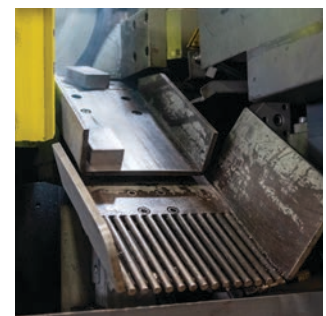
Automatic, hydraulic discharge chute sorts finished pieces
